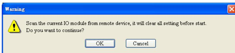
(10) Click on "OK". DeviceNetBuilder will then detect the special module connected to RTU-DNET and the number of points in the DI/DO module and display the information on "RTU Configuration" page.
