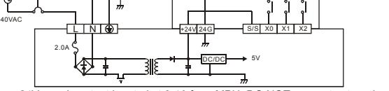
The +24V supply output is rated at 0.4A from MPU. DO NOT connect external power supply to this terminal. Moreover, it takes 5~7mA to drive each input point, so total of 100mA is needed for 16 input points. As a result, the output loads of +24V should not exceed 300mA.
